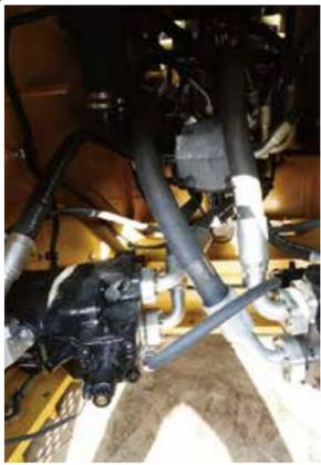
Upgraded hydrostatic system not only leverages Caterpillar automatic, dual path, hydrostatic drive with electronic control technology of the third generation TTT, but also increases efficiency and reliability
